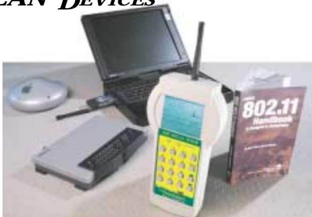
2. Pictured here is Berkeley Varitronics' (Metuchen, NJ) IEEE 802.11 WLAN Grasshopper product. This handheld receiver measures signal strength, bit-error rates (BERs), and even shows multipath energy. Additionally, it provides real-time display of key parameters to enable installers to optimize placement of nodes and identify sources of interference.
