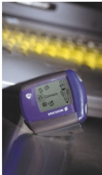
[2] Bluetooth Infowear, a wristwatch that acts as an organizer, synchronizes information wirelessly with a PC.
